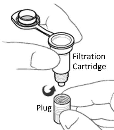
The Plug screws onto the base of the Filtration Cartridge. To ensure a tight seal, give a firm twist by hand.
