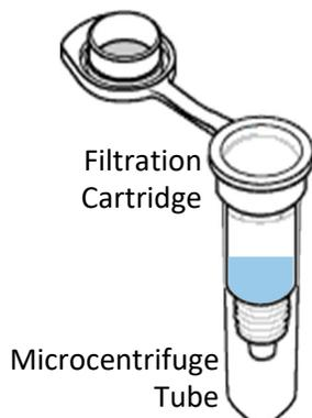
Place the Filtration Cartridge into a Microcentrifuge Tube prior to loading into the centrifuge.
