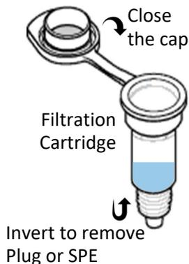
After sample and reagents have been added to the Filtration Cartridge, cap it and invert before unscrewing the Plug or SPE Cartridge.
