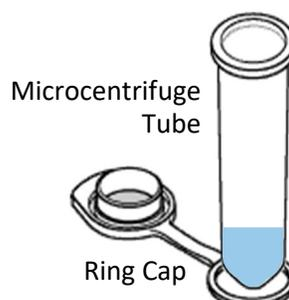
A Ring Cap is provided to conveniently store your sample in the Microcentrifuge Tube. Slide the Ring Cap on to the Microcentrifuge Tube from the bottom.
